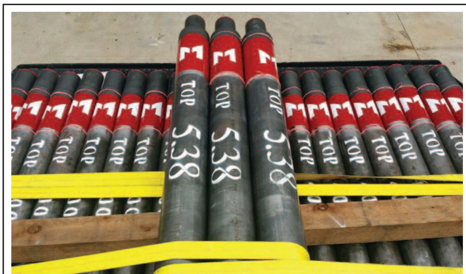
Multilift Welltec LLC's SandGuard™ is a tubing-string tool designed to be installed above an electrical submersible pump to protect it from sand fallback. Instead of sand falling back onto the pump and clogging it, the tool allows the sand to go back into solution and be produced to surface along with the fluid stream.
